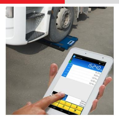
DINI SMART AXLE is a specific tablet/smartphone software, to combine with our <u>WWS axle weighing scales</u>, which allows the weighing of any kind of vehicle in a simple and rapid way. It can also share the data at the same time with the company's IT system. The program offers many functions of weighing, recording and sharing, via ftp, email or other data exchange formats.
